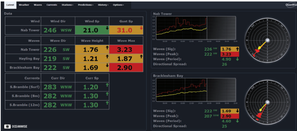
Figure 3: The Pilots page contains environmental data, such as tides, wind, waves, and other metocean data, to help pilots and launch crew make informed and safe decisions regarding marine pilotage.
