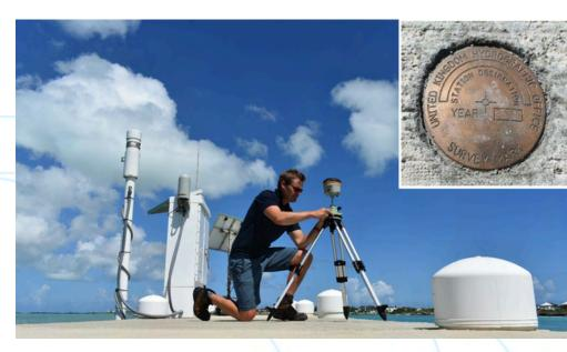
Where required, our team of engineers undertake Global Navigation Satellite Systems (GNSS) surveys to establish geodetic marks for tide gauge levelling and establishing a local datum.
